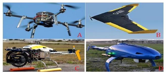
Figure 1: Types of drones currently in use: A (Multi Rotor), B (Fixed Wing), C (Single Rotor) and D (Hybrid VTOL). *Source*: CircuitsToday, 2018.
