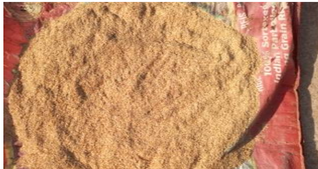
Figure 1: Prepared rice husk for experiment Source: Nigerian Building and Road Research Institute Laboratory
