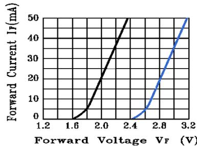
Figure 6: Forward current vs forward voltage.
