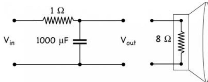
**Figure 7:** Low-pass audio filter
