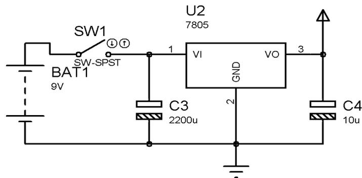
**Figure 1:** Power supply circuit diagram
