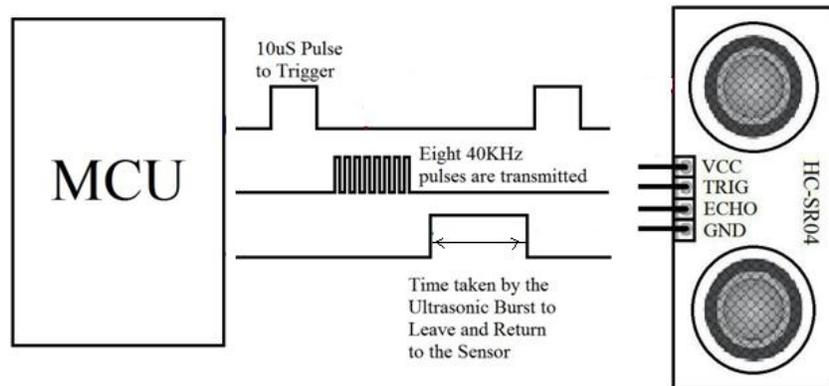
**Figure 3:** Ultrasonic timing control
