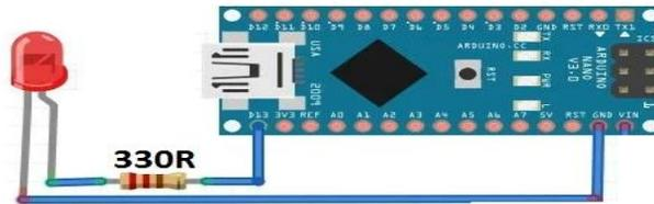
Figure 5: ATmega328p circuit connection with LED
