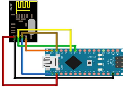
**Figure 8:** Arduino single board interfaced with nRF24L01
