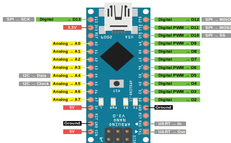
**Figure 2:** Arduino Nano (Single board)
