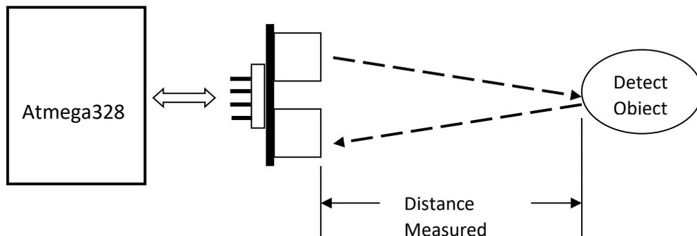
**Figure 4:** Ultrasonic working principle
