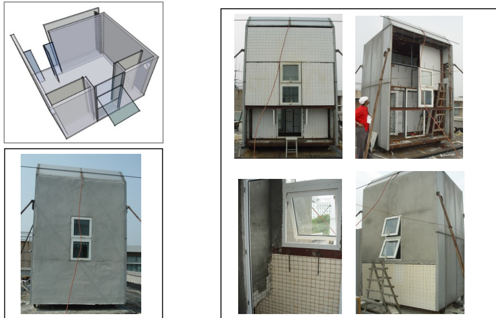
Figure 7: Images of the Ventilated Cavity Wall experimental model (Source: Author's physical model)
