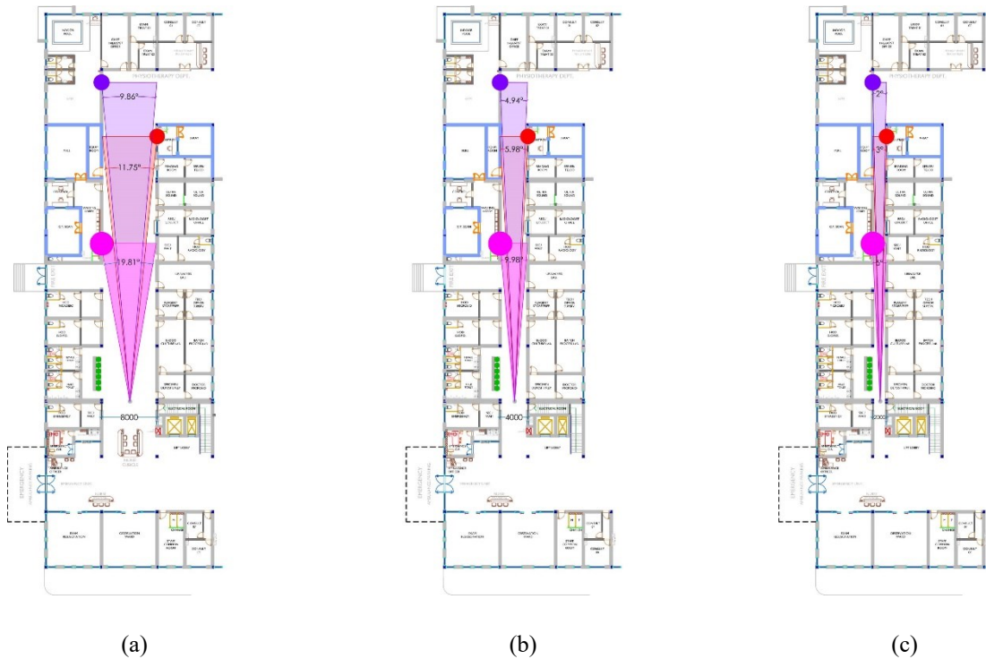
Figure 16: Comparing the view shed and visibility angles for (a) the 8m circulation corridor, (b) the 4m circulation corridor, and (c) the 2m circulation corridor
