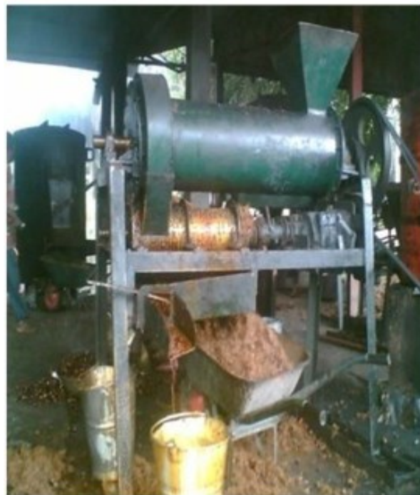
Figure 8: Mechanical method of removing palm fruits mesocarp from endocarp.
