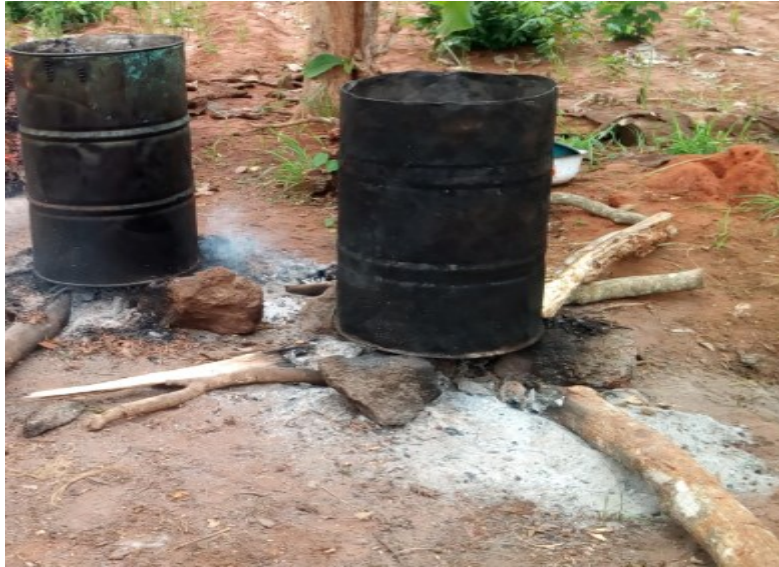
Figure 10: Obtaining refined palm oil from heating of crude palm oil
