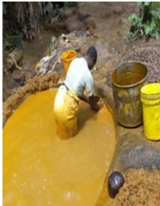
Figure 9: Local way of separating palm oil from other constituents
