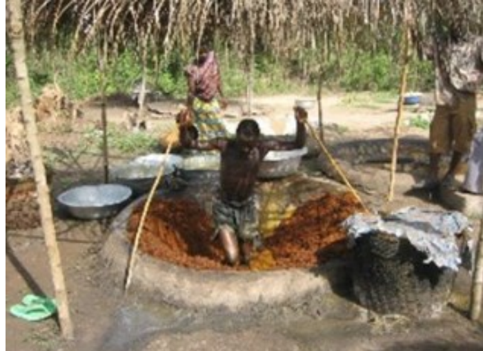
Figure 7: Traditional method (the use of leg) of grinding palm fruits to remove mesocarp from endocarp
